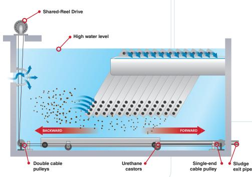
Side view of MRI Hoseless Cable-Vac shows the low profile design. This enables use under plate settlers or tube settlers where clearance can be limited or in open basins.
