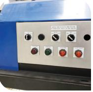
The Integrated Local Control Module (ILCM) is built into the collector drive. This option offers many of the same capabilities as a PLC/HMI and is a costeffective alternative.
